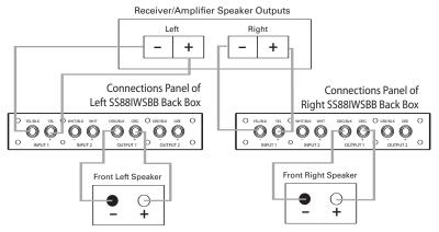
The SS88IWS's onboard crossover feeds the low-passed signal (2nd order at 100Hz) to the SS88IWS subwoofers, and the high-passed signal to the speaker-level outputs for connection to the satellite speakers.
